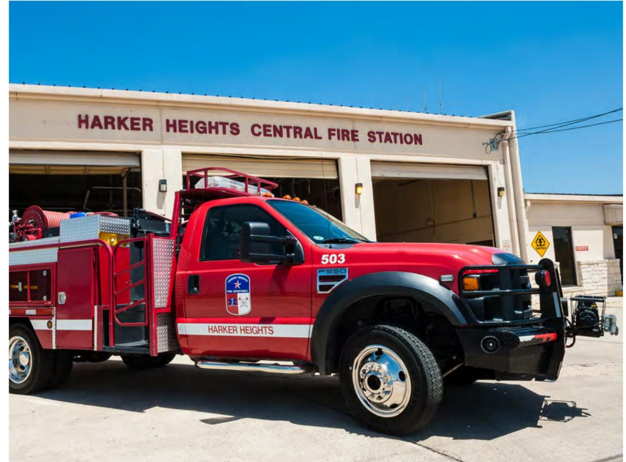
Brush Trucks are designed to move quickly through areas that other fire apparatuses cannot. They can store up to 400 gallons of water and can be used for light rescue, initial attack or medical support.
