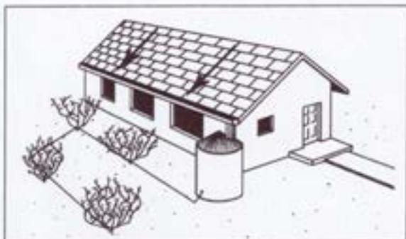
Complex water harvesting system with roof catchment, gutter, downspout, storage and drip distribution system.
